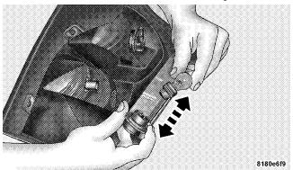
Removing Bulb From Socket
